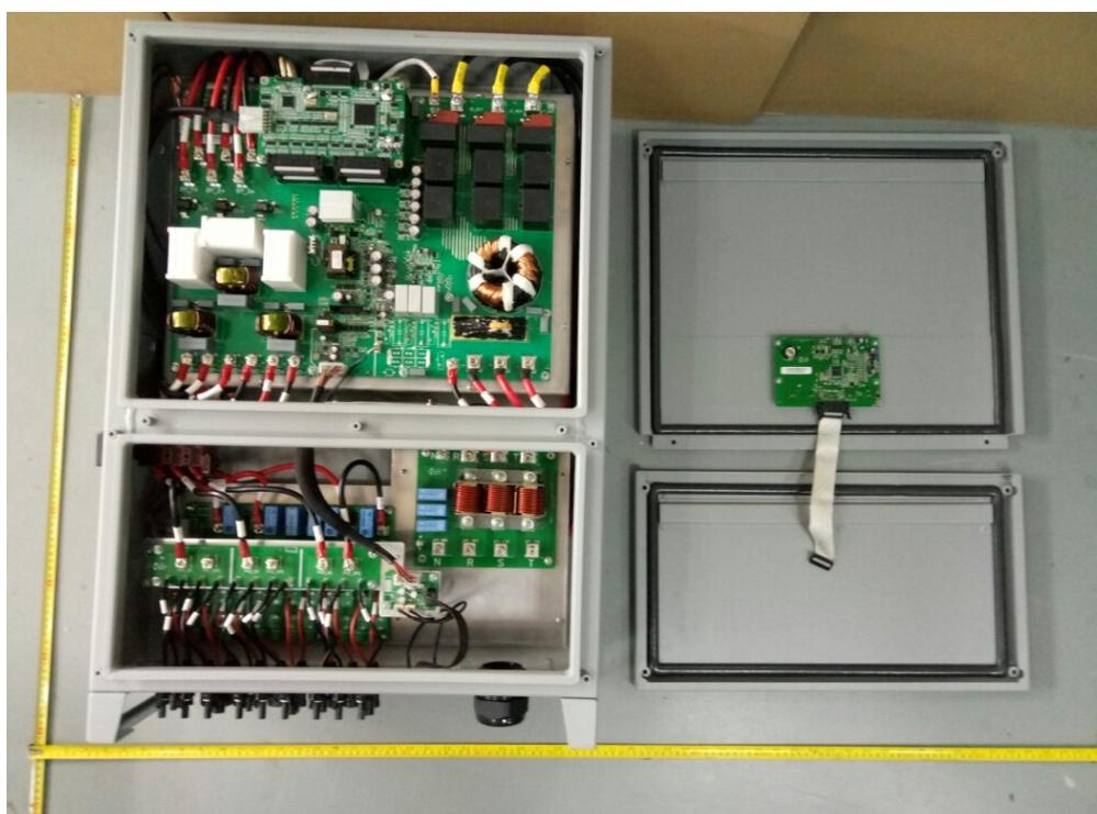
Figure 8. Internal view for Suntrio Plus 60K
