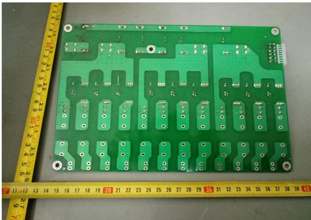
Figure 21. Input board solder side view for Suntrio Plus 60K
