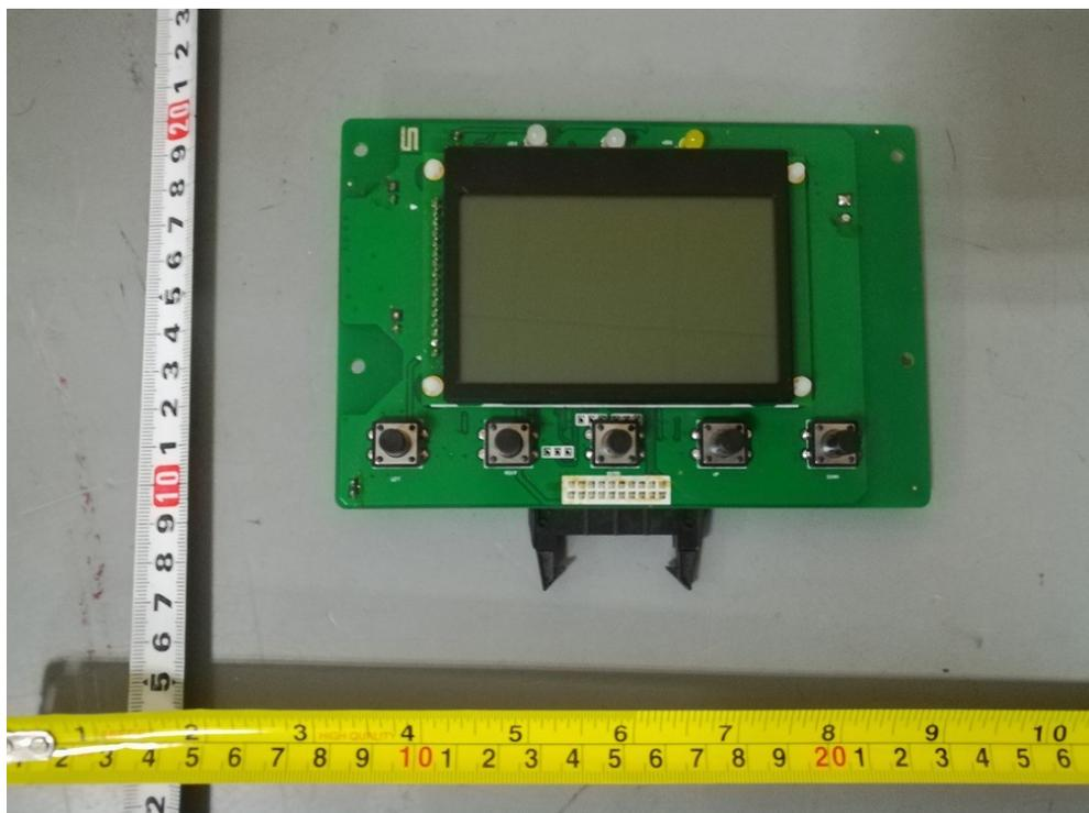
Figure 14. Display board component side view
