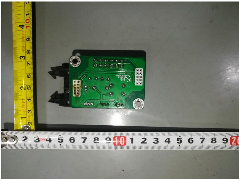
Figure 25. communication board solder side view
