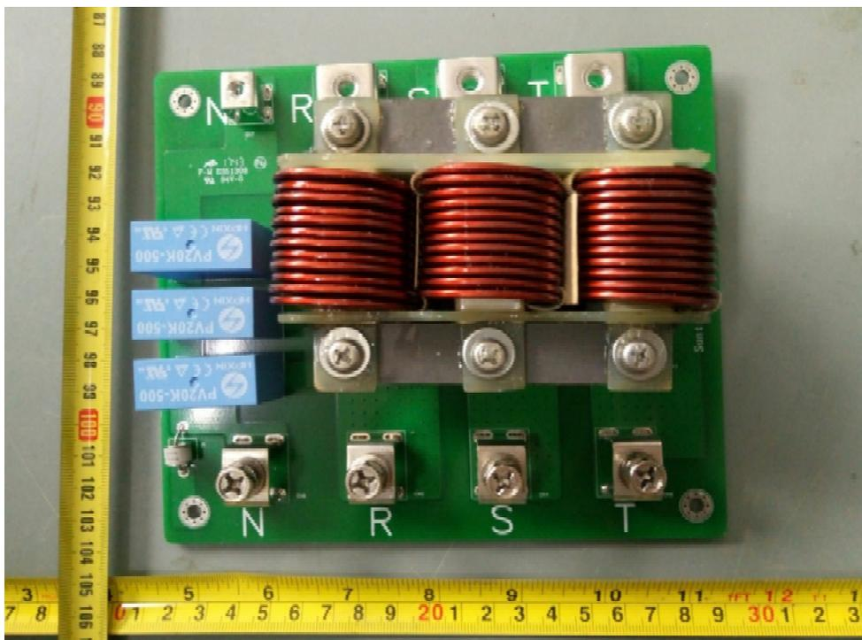
Figure 26. AC board component side view
