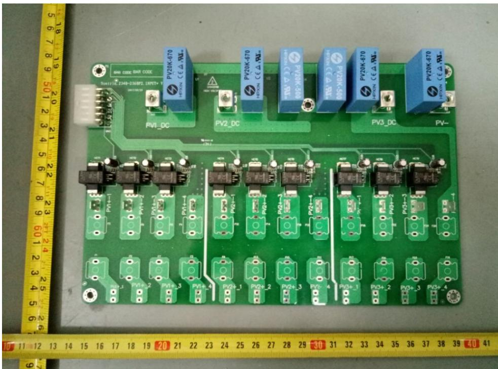
Figure 20. Input board component side view for Suntrio Plus 60K
