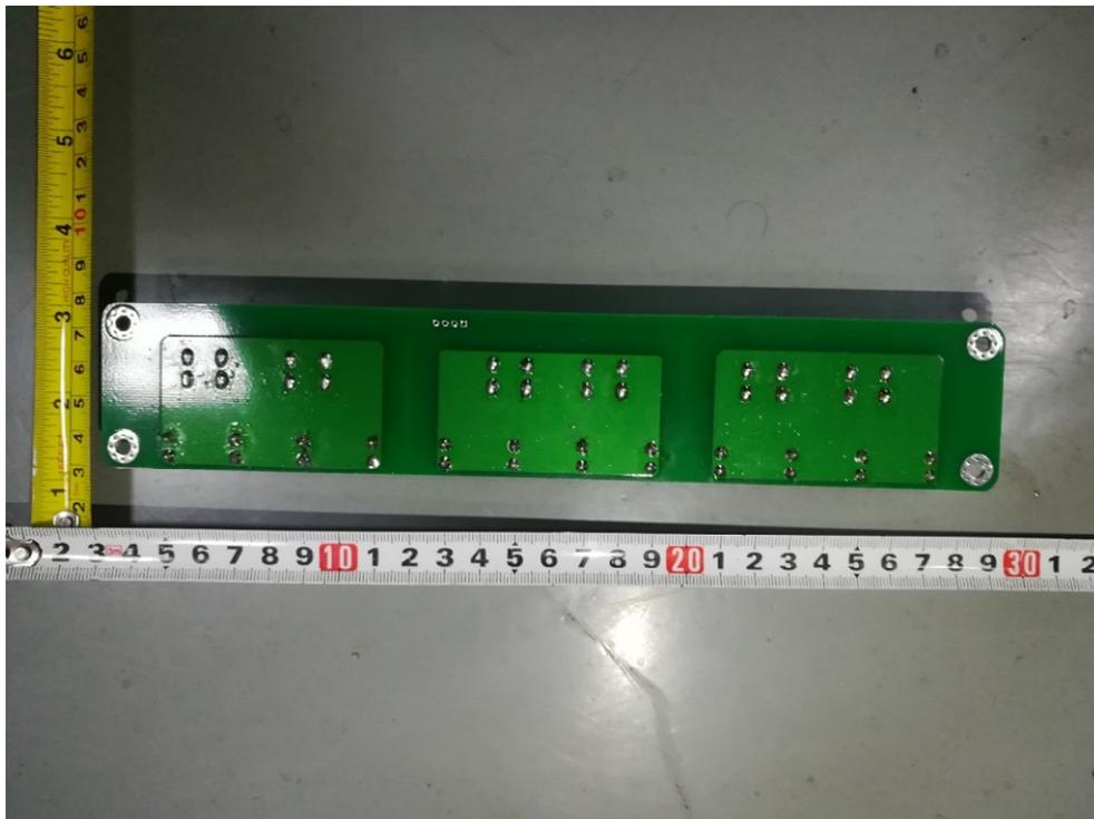
Figure 19. Input board solder side view
