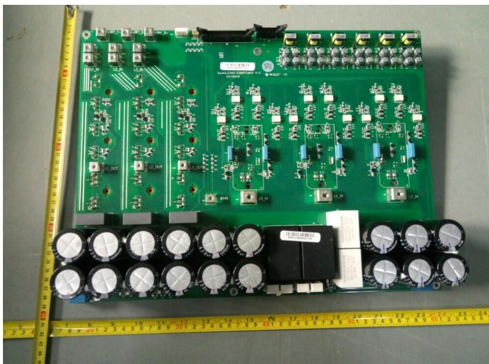
Figure 12. Main power board component side view
