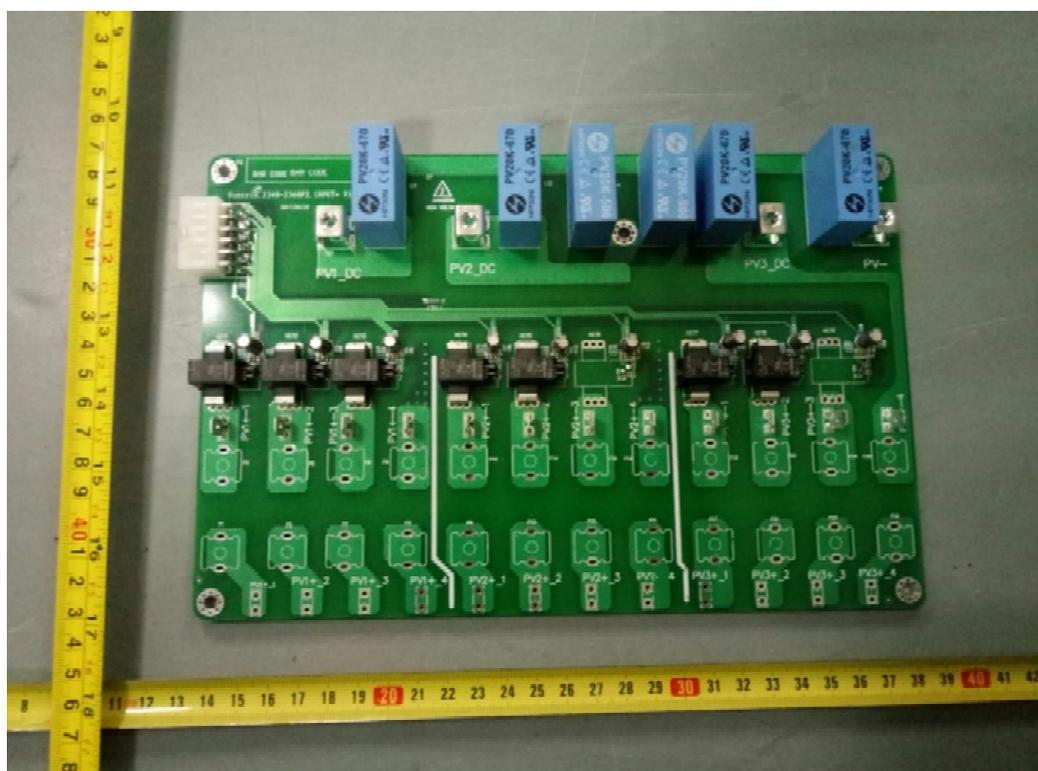
Figure 22. Input board component side view for Suntrio Plus 40K, Suntrio Plus 50K
