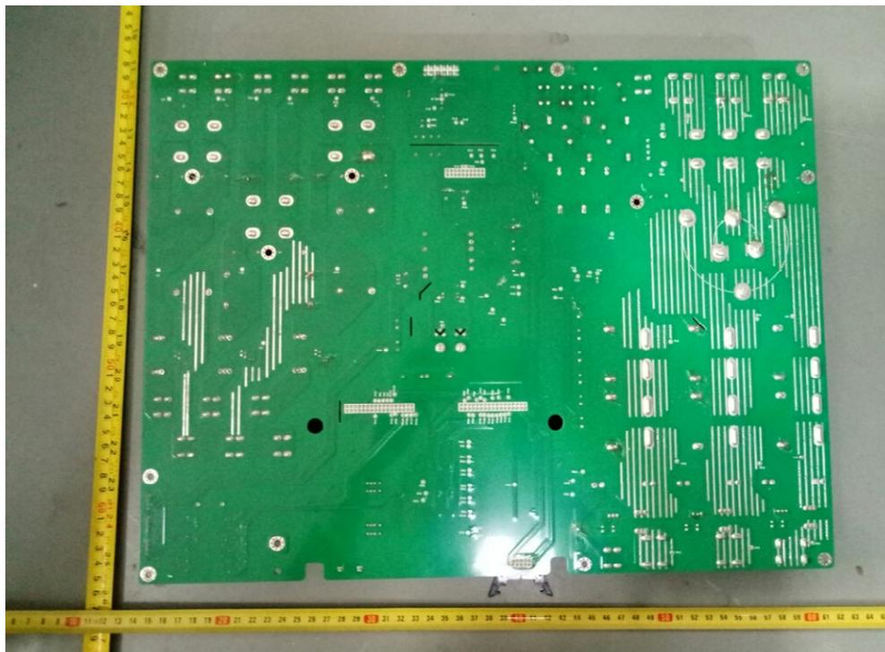
Figure 11. Input/output board solder side view
