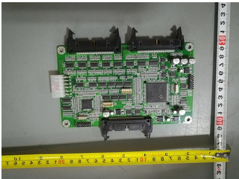
Figure 16. Control board component side view
