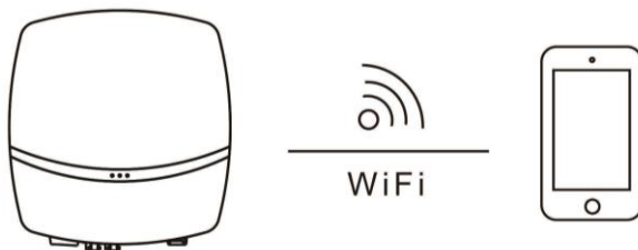
Figure 6.7 Wi-Fi connection schematic diagram
