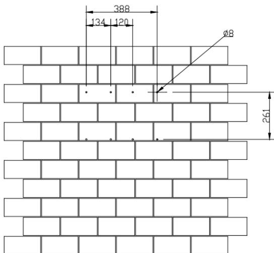
Figure 4.8 Drill Holes (Suntrio Plus 40K/50K/60K)
