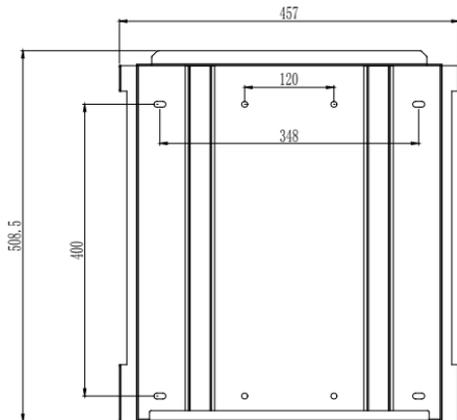
Figure 4.3 Dimensions of rear panel Suntrio Plus 12K/15K/17K/20K
