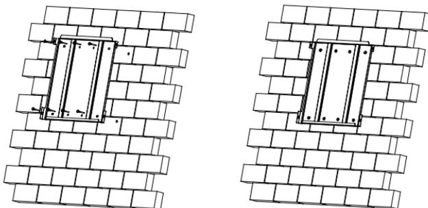
Figure 4.9 Mount the rear panel
