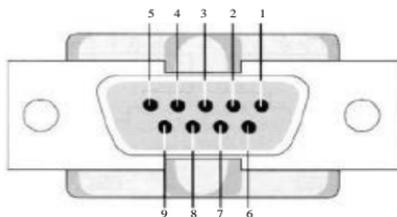
Figure 5.10 Pins of nine serial port cable
