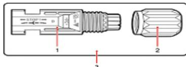
1. Insulated Enclosure      2. Lock Screw      3. Negative Connector
