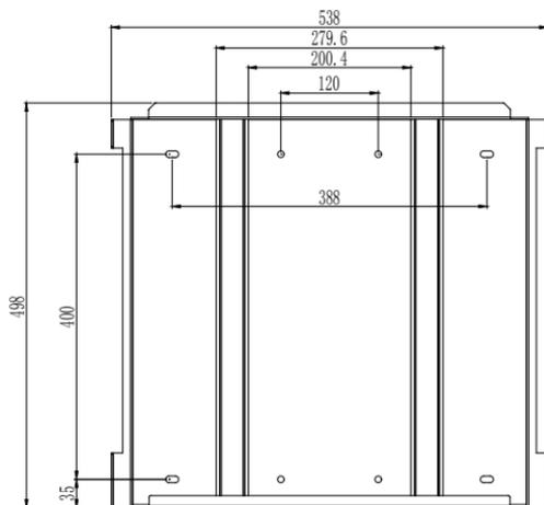
Figure 4.4 Dimensions of rear panel Suntrio Plus 25K/30K/33K
