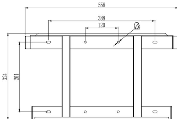
Figure 4.5 Dimensions of rear panel Suntrio Plus 40K/50K/60K
