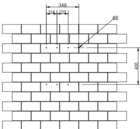
Figure 4.6 Drill holes (Suntrio Plus 12K/15K/17K/20K)
