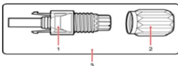
1. Insulated Enclosure      2. Lock Screw      3. Positive Connector
